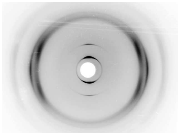
Fig. 8. Image plate X-ray photograph of a PBO3O4 fibre, acquired at room temperature. Stretching direction vertical.
